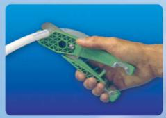
Cutting the pipe is easy, just use a simple tool such as shear or pipe cutter.
